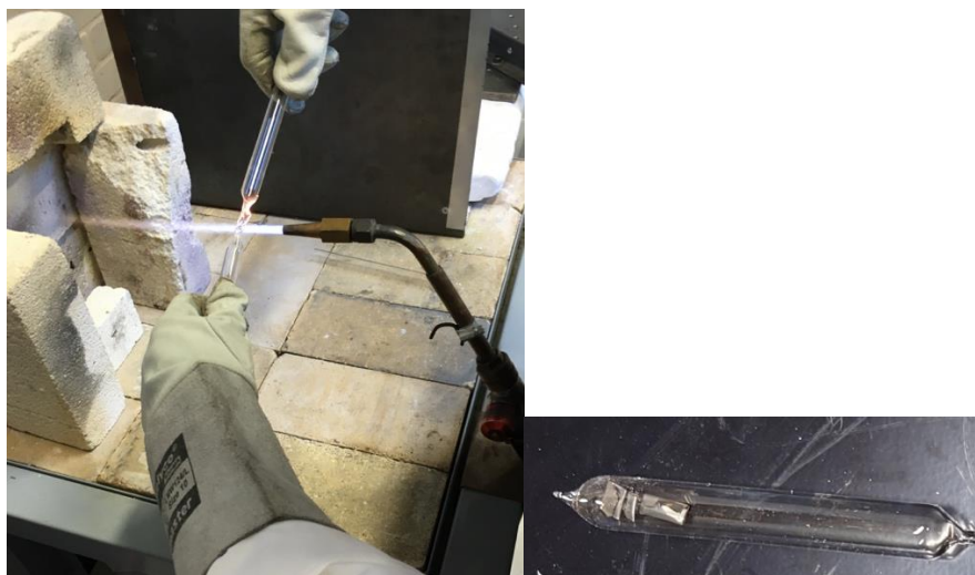
Figure 4 - Encapsulation into a quartz tube and back filled with argon.
